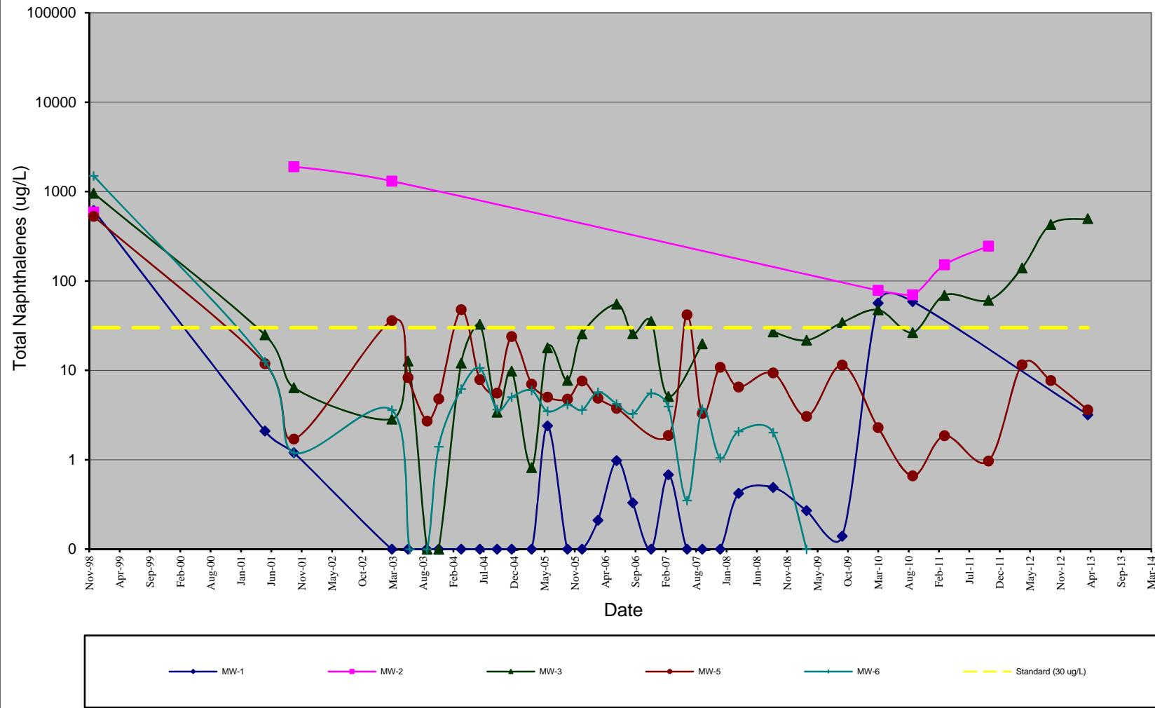
**Figure 4-2B. BNSF Albuquerque - Historical Total Naphthalene Concentrations
