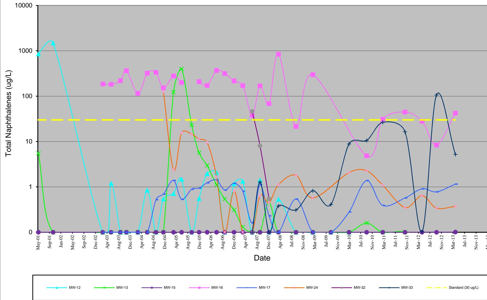
**Figure 4-2D. BNSF Albuquerque - Historical Total Naphthalene Concentrations
